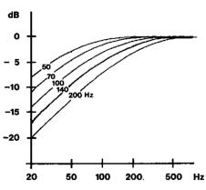
If your satellites are properly damped at the bass resonance — as shown in curve "a" below — the knob should be selected to the same frequency as was set for the Subwoofer upper frequency limit in 6 B. If your satellite speakers are underdamped ("boomy"), the knob should be set to a higher frequency and if they are overdamped ("dry") a lower setting is best.
