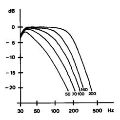
between the preamp and power amp as in 4 A – which is recommended – the knob should be set to 100 Hz if your satellites have decent bass. However, if they have a resonance frequency above 70 Hz, the subwoofer should work higher up.
