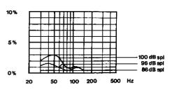
Typical distorsion at different output levels. 2nd + 3rd harmonics.
